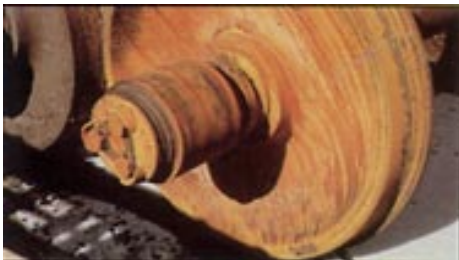
Fig. 5 : Wheel & bearing assembly showing evidence of excessive heat.
