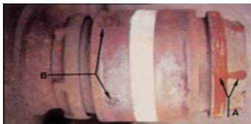
Fig. 9 : Adapter has been displaced to outboard end of bearing. Thrust shoulders has been riding on the end cap flange and rim (A) and has also been point loading the outer race at two points (B)
