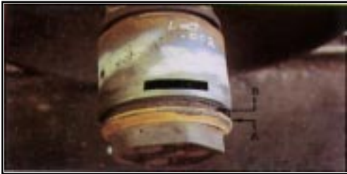
Fig 13: Adapter has been displaced to outboard end of bearing and has cut away the end cap flange (A) and grease seal case (B). This condition would require inspection from the side of the bearing to be detected. Inspection from the end of the bearing would not reveal the damage.
