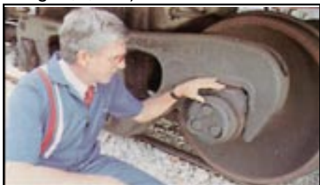
Fig.6 : Adapter properly positioned in side frame
