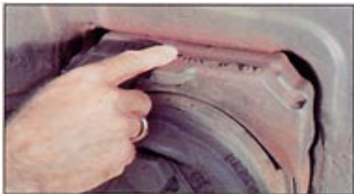
Fig. 8 : Adapter crown (cast) relief area
