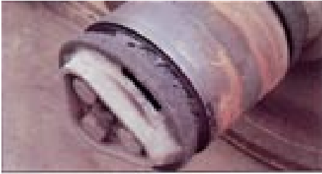
Fig.14: Grease leaking between cup counter bore and grease seal case
