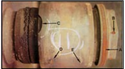
Fig. 11: Adapter has been displaced to outboard end of bearing. Thrust shoulders have been in contact with end cap flange (A) and rim (B) have broken the cup counter bore (C). At one time the adapter was also correctly positioned as indicated by contact patterns on cup outside diameter.
