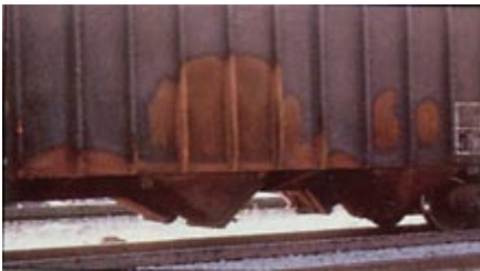
Fig. 3 : Car body showing heat damages.
